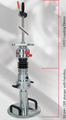
50 mm CBR plunger with handles, adapter disk, housing pin with acceleration sensor, guide tube for
