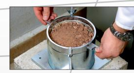
Latch falling weight at upper notch
