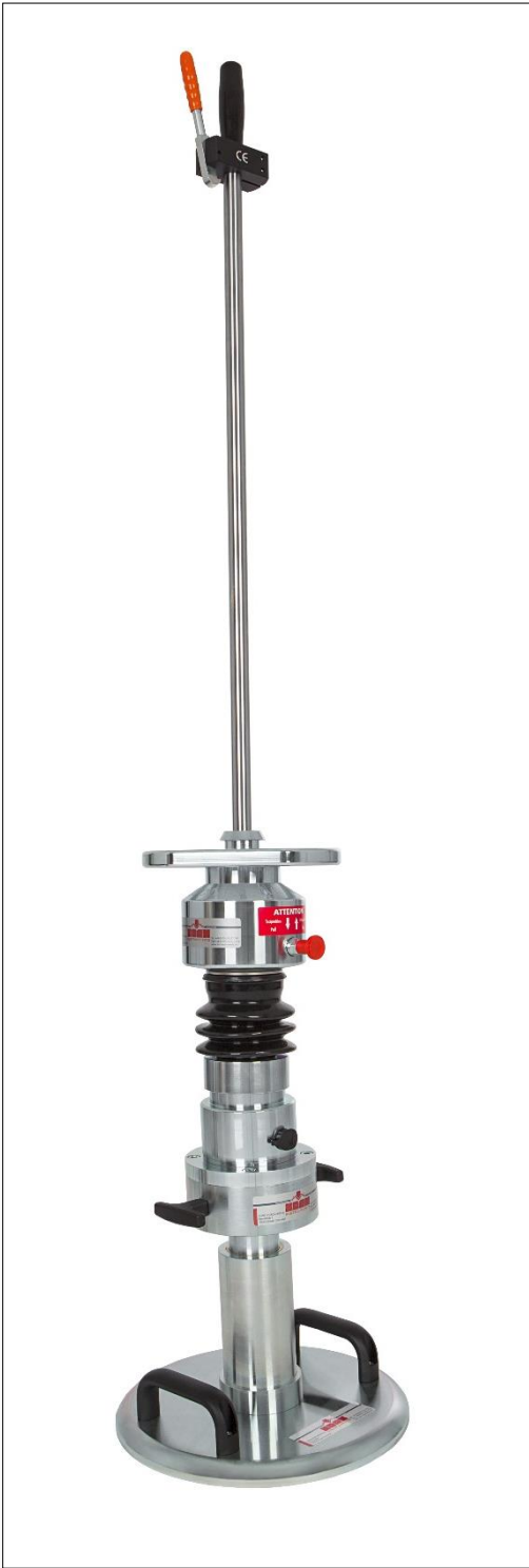
Picture 1: Complete assembly of the CBR-field test with Static force application device with 10 kg drop weight
