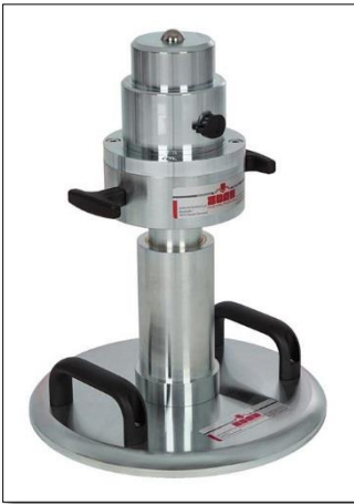
Picture 7: Complete assembly of CBR field test
