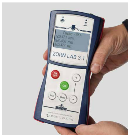
Picture 5 Automatic data acquisition with electronic LWD controller. (e.g. ZORN ZFG 3.1)
