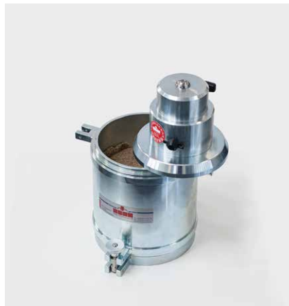
Picture 2 ZORN LAB LWD load plate placed on specimen surface
