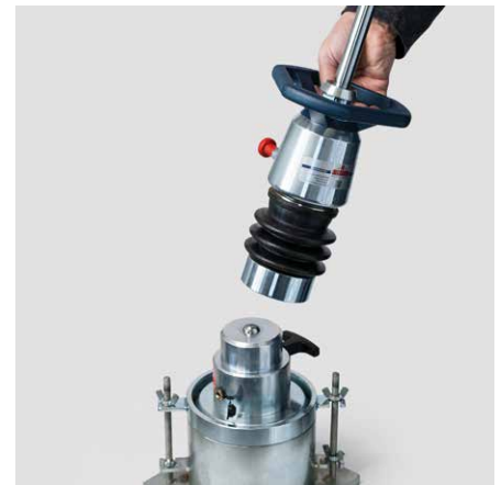
Picture 3 ZORN LAB LWD loading device positioned on the load plate
