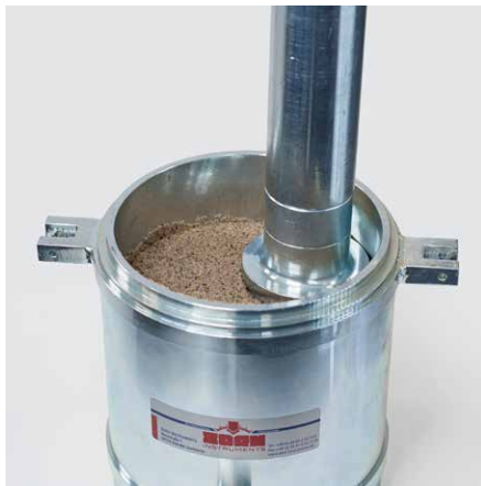
Picture 1 Specimen of compacted soil or soil-aggregate in 6-inch Proctor mould
