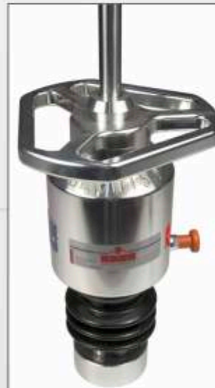
15 kg falling weight for an extended measuring range (Evd 70 - 105 MN/m 2 )
